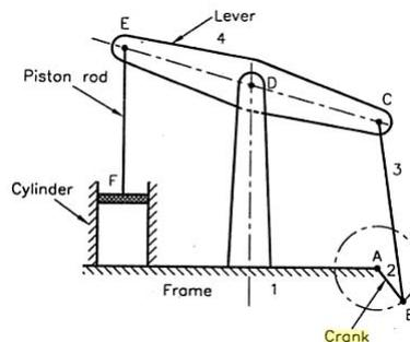
Figure 4.1: Beam engine
