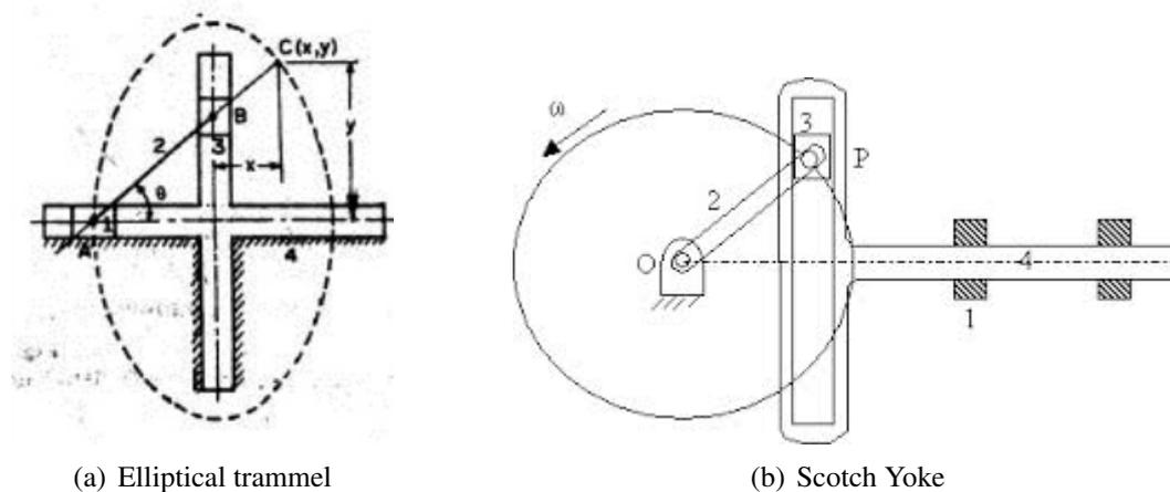
**Figure 4.2: Inversions of double slider crank chain**
