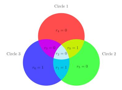
Clearly, Circles 2 and 3, in the figure above, have even numbers of 1's, but Circle 1 does not. We conclude that the error cannot be in Circles 2 and 3, because their rules are satisfied. So it must be  $r_4 = 0$  that is in error. Thus,  $r_4$
