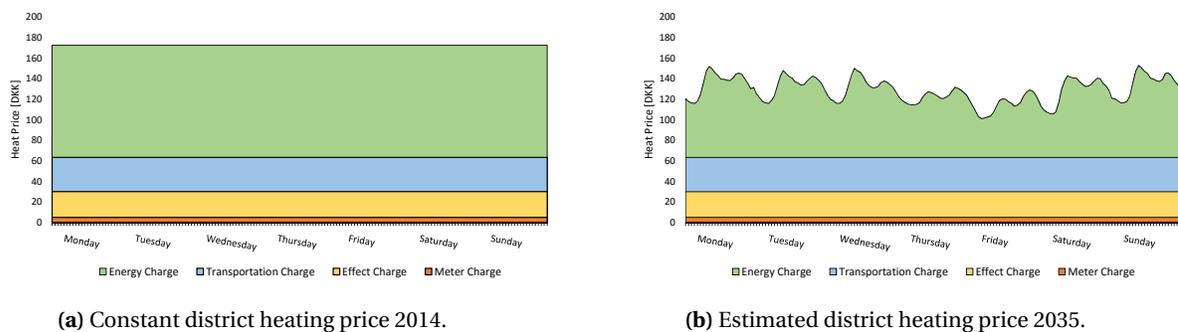
**Figure 3:** Illustration of the various parts of the heat price in 2014 and in 2035. The charges are accumulated and are calculated as an average weekly price throughout the course of a year for a household of 130 m<sup>2</sup>. [13]
