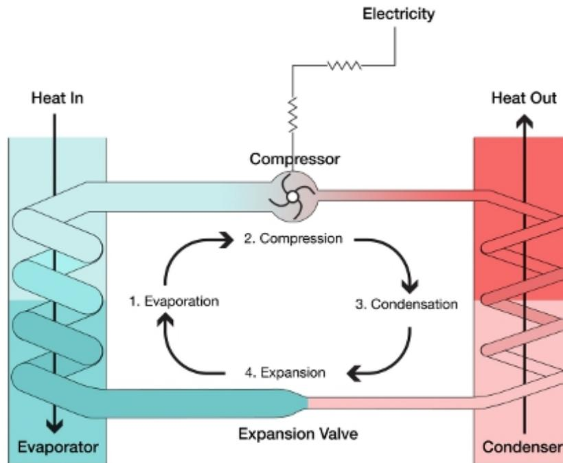
Figure 5: Compression and expansion cycle of a heat pump. [16]
