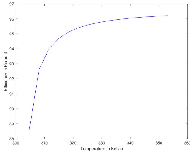
**Figure 10:** Storage efficiency as a function of temperature in each storage layer. The maximum and minimum temperatures are 80°C and 31.5°C, respectively.
