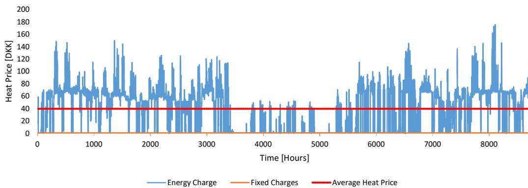
**Figure 11:** Illustration of the hourly district heating price. The fixed charges, the orange line, are so low on an hourly basis, that they do not have an effect on the total price. The red line illustrates the average district heating price.
