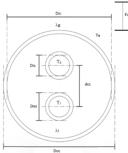
**Figure 14:** Schematic of a Twin-pipe district heating transmission pipe [26].
