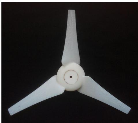
Fig. 16. Printed upper rotor
