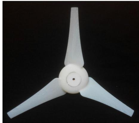
Fig. 17. Printed lower rotor
